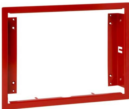
The VES trim ring allows the eVIEW annunciator to easily be recess mounted. VES trim rings provides placement tabs that fold behind dry wall. Traditional screw mounting is available by 2 openings in each of the vertical frames. Conduit entry is not blocked by trim ring.
